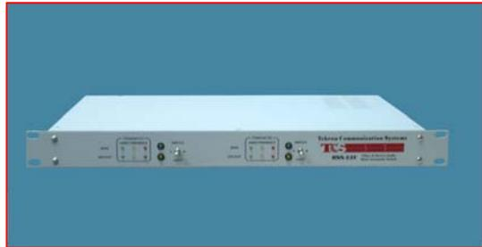
Each switch module in the chassis can accept two video/audio input channels to switch automatically to the backup input channel when Video-freeze condition is detected, or either the main input video Sync or both Left & Right audios drop below their respective Threshold level setting. The RSS will switch back automatically to the main input after the faulty signal is restored to a level above its threshold setting.
